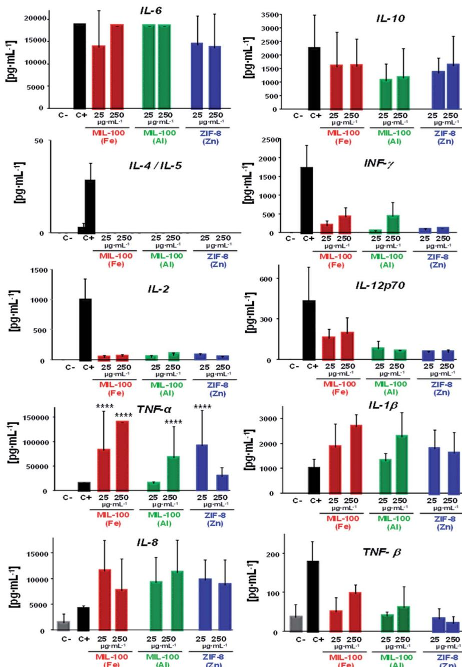
Fig. 3 Individual levels of human cytokines production from peripheral blood mononuclear cells (3 different donors) after 24 h in contact with 25 or 250  $\mu\text{g mL}^{-1}$  of MIL-100(Fe), MIL-100(Al) or ZIF-8(Zn) NPs. C-: negative control (PBS) and C+: positive control (10  $\mu\text{g mL}^{-1}$  PHA + 1  $\text{mg mL}^{-1}$  LPS). All data were tested by two-way ANOVA and Tukey's tests ( $P < 0.05$  was considered statistically significant).
