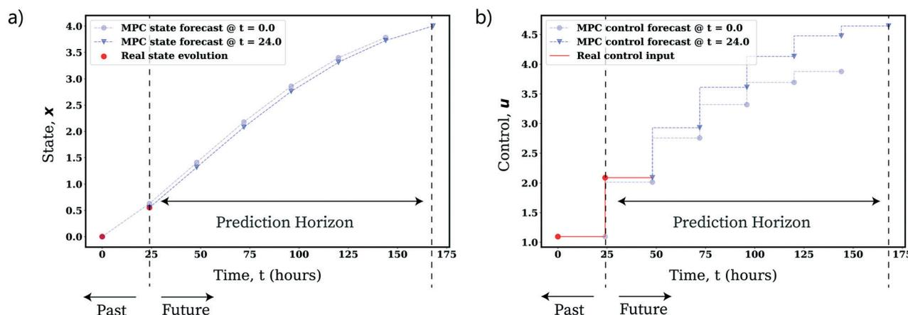
**Fig. 30** Demonstration of the use of state-feedback in receding horizon MPC for online optimization of an uncertain, nonlinear fed-batch process. Optimized forecast and evolution of a) the state trajectory, b) the control trajectory (composed of piecewise constant control inputs). See ref. 158 and 159 for more information on the system detailed.
