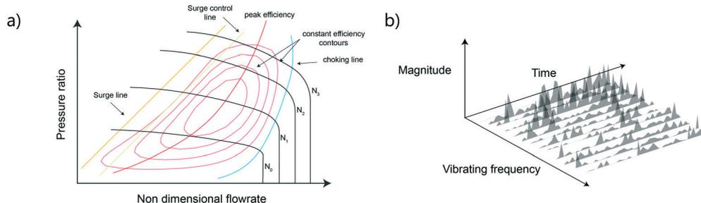
**Fig. 16** Compressor characteristic (a) and spectrogram (b) are two traditional approaches to detect inefficient or anomaly operating modes. These calculations can be considered feature engineering to be combined with statistical or machine learning methods.
