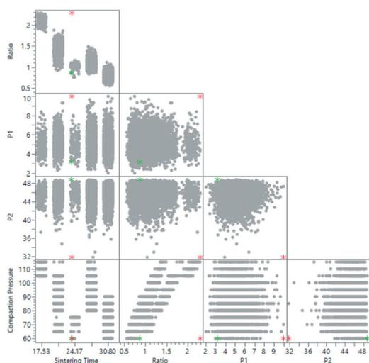
**Fig. 14** Scatterplot matrix showing historical data of a manufacturing process where the optimal prediction point is shown without extrapolation control (red) and with extrapolation control (green). A boosted neural network was previously trained to predict failure and quality. The reader is referred to ref. 60 for a detailed discussion.
