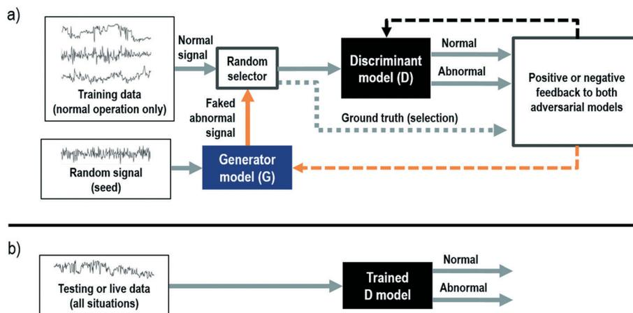
**Fig. 15** This figure shows a simplified schematic representation of training (a) and use (b) of generative adversarial networks (GANs) for anomaly detection on time-series data. Generator (G) and discriminant (D) models are trained through iterations based on the performance feedback of the D model. Both models compete until satisfactory performances are achieved. Then, D model can be used as an online classifier for anomaly detection, bottom scheme.
