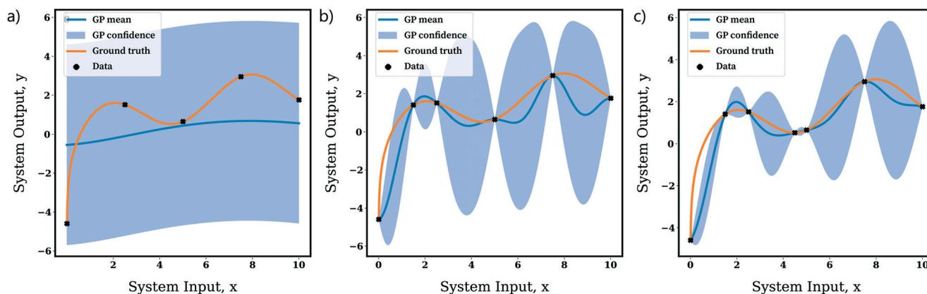
**Fig. 28** Expression of a Gaussian process posterior (*i.e.* its mean and uncertainty predictions) for the modeling of a smooth noiseless function. The figure demonstrates the effects of an increasing number of data points: a) 5 data points, b) 6 data points, c) 7 data points. Note how as the number of data points increases, the uncertainty estimate (*i.e.* the 95% confidence interval) reduces and the mean GP prediction becomes a better estimate of the ground truth.
