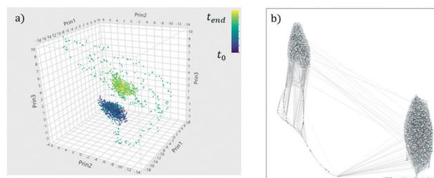
**Fig. 12** A transition between two steady-state regimes for the Tennessee Eastman process (simulated data<sup>49</sup>) visualized with (a) PCA and (b) UMAP.<sup>52</sup> UMAP is able to better reduce the number of tags into two dimensions. The reader is referred to ref. 51.
