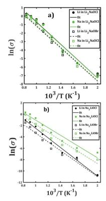
Fig. 7 Arrhenius-type dependence of Li and Na dc-conductivity of (a)  $\text{Li}_2\text{NaOX}$  and (b)  $\text{Na}_2\text{LiOX}$  nanocrystalline sample.
