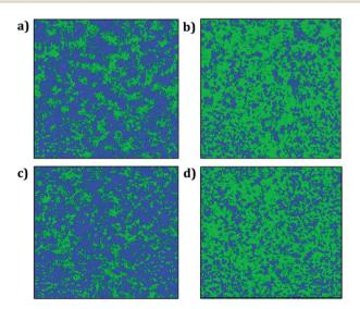
Fig. 8 Trajectory plots of Li and Na in (a) Li<sub>2</sub>NaOCl, (b) Na<sub>2</sub>LiOCl, (c) Li<sub>2</sub>NaOBr and (d) Na<sub>2</sub>LiOBr compounds after 2 ns. Blue and green lines represent the Li and Na trajectory lines, respectively.
