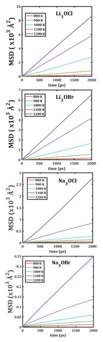
Fig. 2 Mean square displacement versus simulation time of each A<sub>3</sub>OX nanocrystalline sample.
