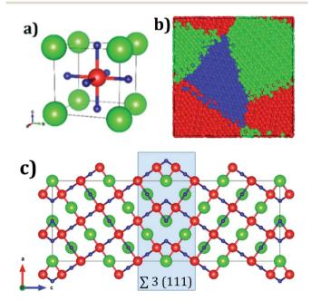
Fig. 1 (a) Unit cell of  $A_3OX$  ( $A=Li^+$ ,  $Na^+$ ,  $X=Cl^-$ ,  $Br^-$ ) lattice structures, green, red and blue represents  $X^-$ ,  $O^{2-}$  and  $A^+$  ions respectively, (b)  $A_3OX$  nanocrystal with three grains, and (c)  $\sum 3(111)$  grain boundary, where the shaded square highlights the grain boundary region. Color coding in (b) represents a unique grain.
