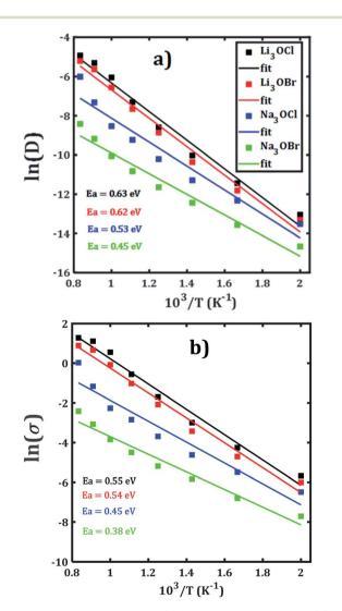
Fig. 3 Arrhenius dependence of (a) diffusion coefficient and (b) DC conductivity of each  $A_3OX$  nanocrystalline samples.
