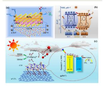
Fig. 13 (a) 2D/2D ReS<sub>2</sub>/CCN heterojunction. Reproduced from ref. 63 with permission from Elsevier, Copyright 2022. (b) Built-in electric field formed by the heterojunction. Reproduced from ref. 144 with permission from Elsevier, Copyright 2020. (c) Schematic mechanism of CN/ CTF heterostructure for photocatalytic CO2 reduction. Reproduced from ref. 145 with permission from the Chinese Academy of Sciences, Copyright 2022.
