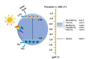
Fig. 1 Schematic diagram of photocatalytic CO<sub>2</sub> reduction over a semiconductor.
