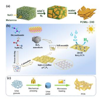
Fig. 4 (a) Illustration of the synthesis process of PCNNs-IHO by onsurface polymerization. Reproduced from ref. 62 with permission from Wiley-VCH, Copyright 2021. (b) Schematic illustration of constructing crystalline g-C<sub>3</sub>N<sub>4</sub> by salt template method. Reproduced from ref. 63 with permission from Elsevier, Copyright 2022. (c) Schematical illustration of microwave thermolysis of urea pellets. Reproduced from ref. 42 with permission from Elsevier, Copyright 2021.
