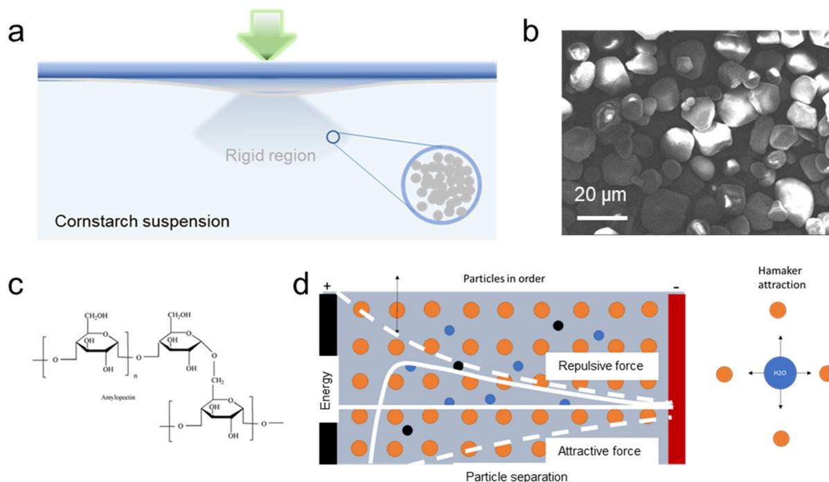
**Fig. 1** (a) Schematic diagram of the cornstarch shear-thickening electrolyte; (b) a SEM image of cornstarch particles; (c) cornstarch molecular structure; (d) a schematic diagram of Hamaker attraction in the suspension.
