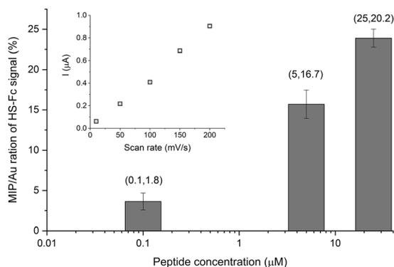
**Fig. 3** Ratio of the anodic peak currents of the surface confined HS-Fc for the MIP after template removal and the respective bare gold surface as a function of the concentration of the G-Peptide template used for immobilization. Please note the logarithmic scale of the X axis. Inset: Scan rate dependence of the surface confined HS-Fc anodic peak current for the MIP made using a 5  $\mu$ M G-Peptide template.
