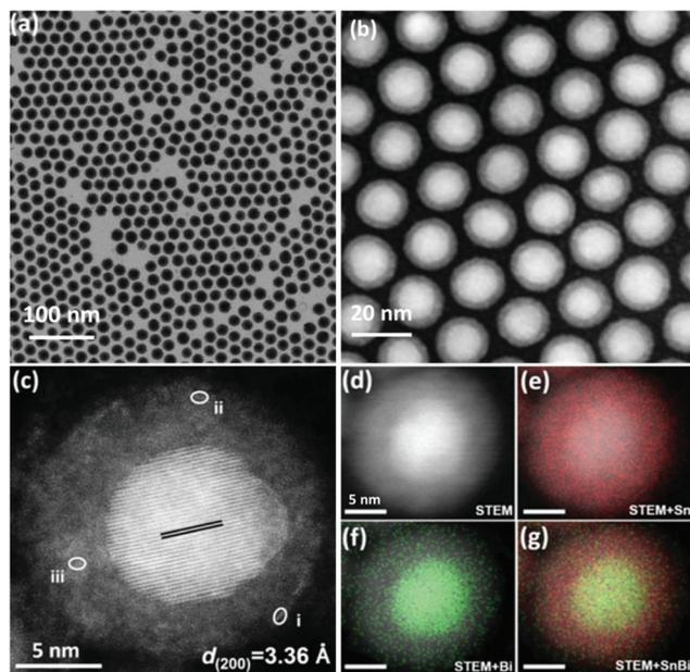
**Fig. 8** (a) TEM, (b) HAADF-STEM, and (c) aberration-corrected HAADF-STEM images of the  $\text{Sn}_{0.80}\text{Bi}_{0.20}$ @Bi-Sn $O_x$  core-shell alloy nanoparticles. (d–g) STEM-EDS elemental mapping images of  $\text{Sn}_{0.80}\text{Bi}_{0.20}$ @Bi-Sn $O_x$  core-shell alloy nanoparticles.<sup>8</sup> This figure has been adapted from ref. 8 with permission from the John Wiley and Sons, copyright 2020.
