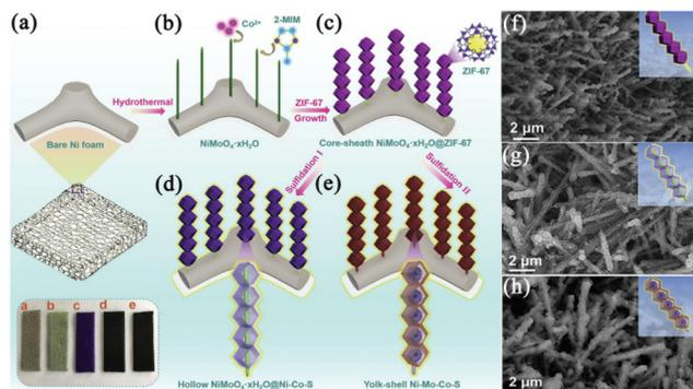
**Fig. 8** (a–e) Schematic illustrations of the synthesis of yolk-shell Ni–Mo–Co–S NCAs on NF. SEM images of (f)  $\text{NiMoO}_4 \cdot x\text{H}_2\text{O}@\text{ZIF-67}$ , (g) hollow  $\text{NiMoO}_4 \cdot x\text{H}_2\text{O}@\text{Ni-Co-S}$  NCAs and (h) yolk-shell Ni–Mo–Co–S NCAs. Reprinted with permission from ref. 98, Copyright 2020, Elsevier.
