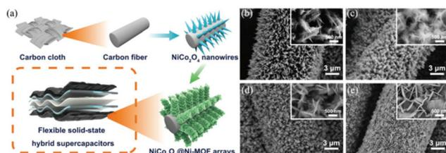
**Fig. 4** (a) Schematic illustration of the synthesis of  $\text{NiCo}_2\text{O}_4@\text{Ni-MOF}$  on CF. (b–e) SEM images of  $\text{NiCo}_2\text{O}_4@\text{Ni-MOF}$  synthesized at 3, 6, 12, and 24 h for MOF growth, respectively. Reprinted with permission from ref. 58, Copyright 2019, American Chemical Society.
