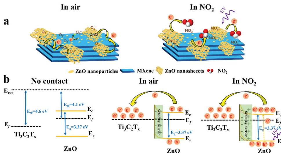
**Fig. 9** (a) Schematic diagram of the possible gas-sensing mechanism of  $\text{Ti}_3\text{C}_2\text{T}_x$ -ZnO NS. (b) Energy band structure diagram of  $\text{Ti}_3\text{C}_2\text{T}_x$ -ZnO NS Schottky barriers in air and  $\text{NO}_2$ .
