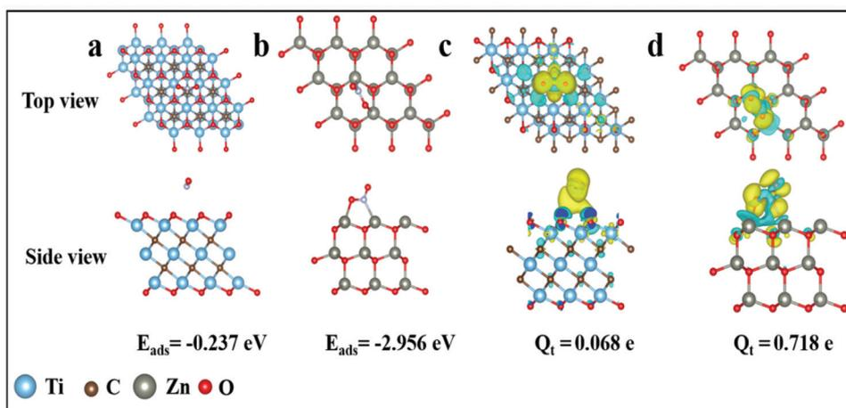
**Fig. 8** Top and side view of the most energetically favorable configuration (a)  $\text{Ti}_3\text{C}_2\text{T}_x$  and (b) ZnO after adsorption of  $\text{NO}_2$  and the difference charge density plots of  $\text{NO}_2$  adsorbed on the (c)  $\text{Ti}_3\text{C}_2\text{T}_x$  and (d) ZnO using an isovalue of  $0.0001 \text{ e}^- \text{ \AA}^{-3}$  and  $0.002 \text{ e}^- \text{ \AA}^{-3}$ , respectively. Cyan: charge depletion. Yellow: charge accumulation.
