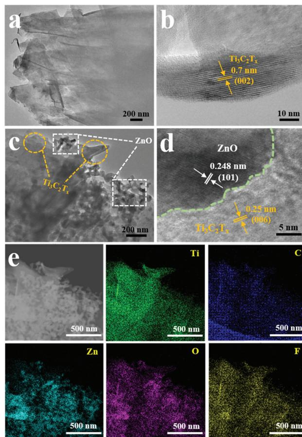
Fig. 5 (a) TEM and (b) HRTEM images of  $\text{Ti}_3\text{C}_2\text{T}_x$ . (c) TEM and (d) HRTEM images of  $\text{Ti}_3\text{C}_2\text{T}_x$ -ZnO NS. (e) The STEM image of  $\text{Ti}_3\text{C}_2\text{T}_x$ -ZnO NS and EDX mapping images of Ti, C, Zn, O and F elements.
