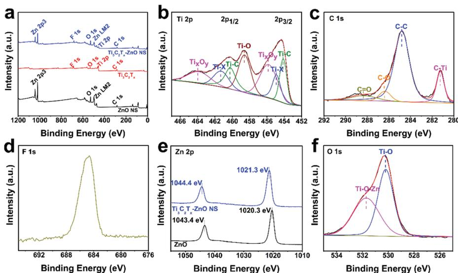
**Fig. 6** (a) Full survey XPS spectrum of  $\text{Ti}_3\text{C}_2\text{T}_x$ , ZnO nanosheets and  $\text{Ti}_3\text{C}_2\text{T}_x$ -ZnO nanosheet hybrids. High-resolution XPS spectra for (b) Ti 2p, (c) C 1s, (d) F 1s, (e) Zn 2p and (f) O 1s of  $\text{Ti}_3\text{C}_2\text{T}_x$ -ZnO nanosheet hybrids.
