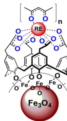
**Fig. 17** Structure of Fe<sub>3</sub>O<sub>4</sub>@calix-Ln( $\beta$ -diketonate). Reprinted with permission from ref. 258. Copyright (2014) American Chemical Society.
