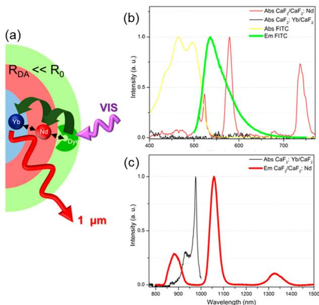
**Fig. 4** (a) Architectural design of  $\text{CaF}_2:\text{Yb}^{3+}/\text{CaF}_2:\text{Nd}^{3+}$  core/shell NP dye-sensitized by **33** and (b–c) spectral overlaps between donor–acceptor emission–absorption bands for multistep sequential energy transfer. Adapted with permission from ref. 103. Copyright 2019, American Chemical Society.
