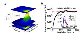
Fig. 4 (a) Time-resolved emission spectra (TRES) of the upconverted fluorescence of the XLG/PVP hydrogel at room temperature under 532 nm laser ([PtOEP] = 10  $\mu$ M, [DPAS] = 2.5 mM). (b) Kinetics acquisition of the UC emission at 442 nm with continuous irradiation of 532 nm laser. The sample has been exposed to ambient atmosphere for 10 days in advance; inset: emission spectra of the UC hydrogel at different irradiation times; ([PtOEP] = 10  $\mu$ M, [DPAS] = 2.5 mM, P.I. = 4.8 mW).
