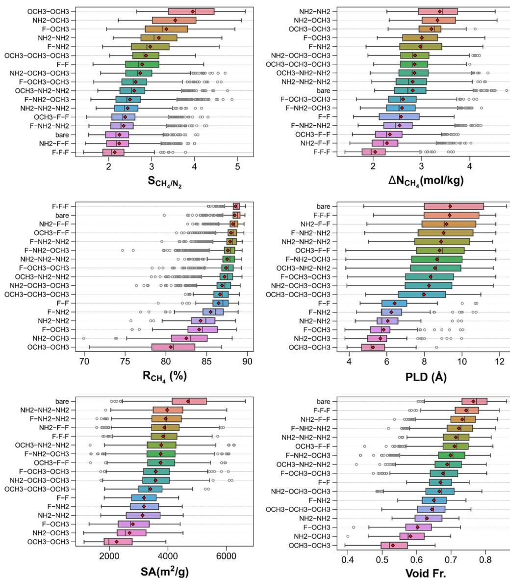
Fig. 5 Breakdown of  $\text{CH}_4/\text{N}_2$  separation performance metrics and textural properties of MOFs.
