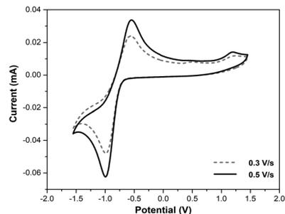
Fig. 2 Solid-state cyclic voltammetry of **Per-MOF** in CH<sub>3</sub>CN using TBAPF<sub>6</sub> 0.1 M as electrolyte at different scan rates. Platinum wire was used as the counter electrode and silver wire as the pseudoreference electrode. Ferrocene was added as internal standard. All potentials are reported *versus* Ag/AgCl.
