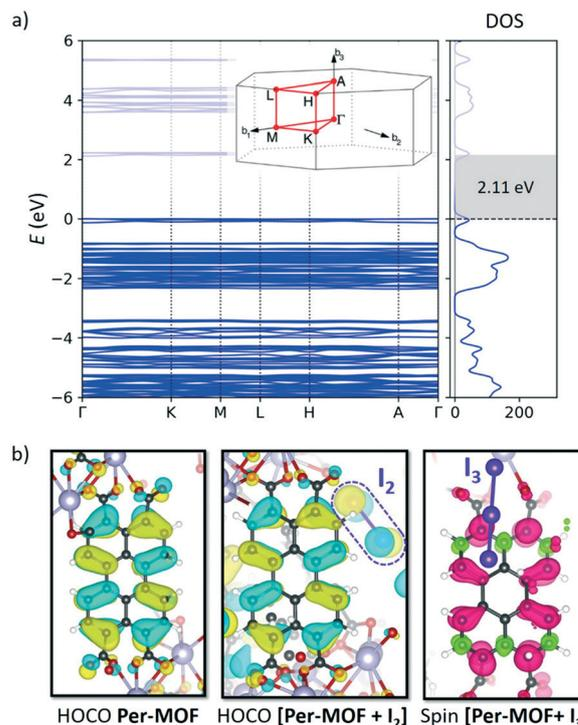
Fig. 4 a) Band structure and density of states (DOS) calculated at the HSE06 level for the full  $k$ -path of the first Brillouin zone of  $P\bar{3}$  space group in **Per-MOF**. The Fermi level was set to the valence band maximum. b) Highest-occupied crystal orbital (HOCO) calculated for evacuated **Per-MOF** and iodine-doped [**Per-MOF** + I<sub>2</sub>], and spin density calculated for [**Per-MOF** + I<sub>3</sub>].
