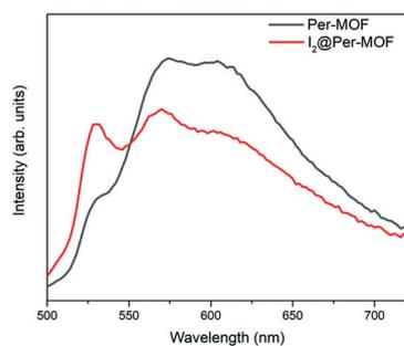
Fig. 3 Solid-state emission spectra of **Per-MOF** and **I<sub>2</sub>@Per-MOF** under 368 nm excitation.
