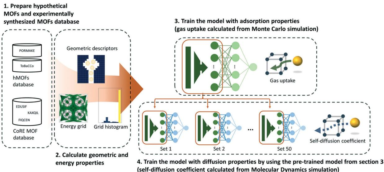
**Fig. 1** Overall schematics of our transfer learning workflow. Two types of MOF databases, hypothetical MOF database (PORMAKE and ToBaCCo) and experimentally synthesized MOF database (CoRE MOF database), were prepared. Geometric properties and energy descriptors obtained from energy grids were used as features for the neural network.
