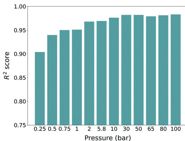
**Fig. 3**  $R^2$  scores of the machine learning models obtained from the source domain (hMOFs and methane gas uptake). All the scores are evaluated from frameworks that are not involved in the data set used during training. All of the models were respectively generated from gas uptakes that were computed at 12 different pressures from 0.25 bar to 100 bar.
