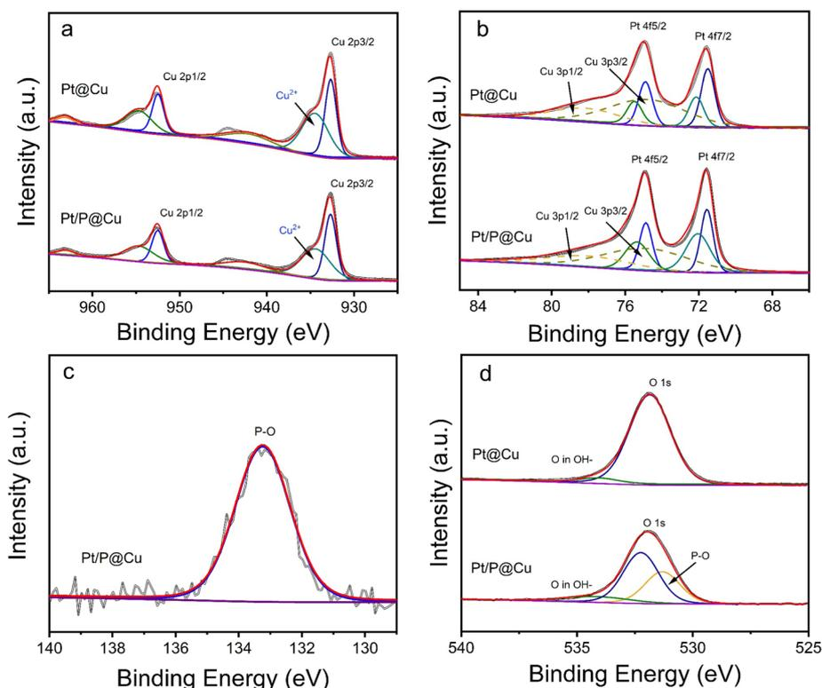
Fig. 3 XPS spectra of (a) Cu 2p, (b) Pt 4f, (c) P 2p and (d) O 1s of Pt@Cu and Pt/P@Cu surfaces.
