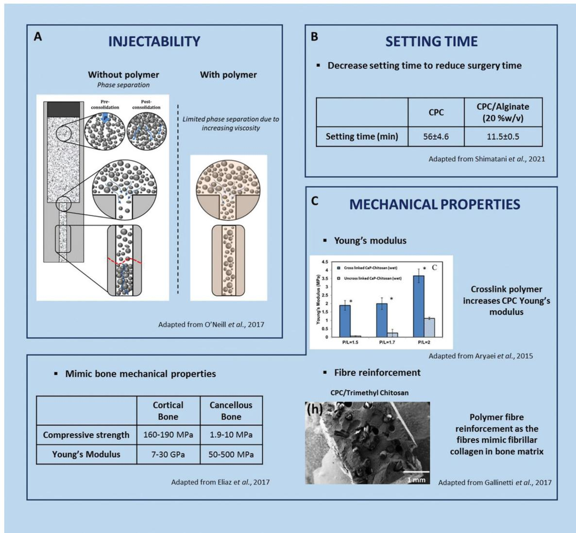
Fig. 5 Improvement of calcium phosphate cement physico-chemical properties by polymer addition.<sup>90,92,93,102,111</sup>
