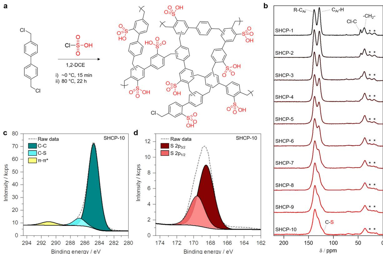
**Fig. 1** Sulfonated hypercrosslinked polymer characterisation. (a) Reaction scheme for the one-pot synthesis of SHCPs. (b)  $^{13}\text{C}$  CP/MAS solid state NMR spectra for all SHCPs, with increasing catalyst to monomer ratio used in the production of SHCP-1–SHCP-10. \* Represents spinning side bands. (c) X-Ray photoelectron C 1s spectrum for SHCP-10. (d) X-Ray photoelectron S 2p spectrum for SHCP-10. (grey dotted lines in (c) and (d) represent raw data).
