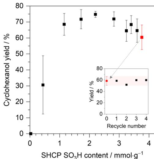
Fig. 4 Cyclohexanol yield of SHCP catalysed hydrolysis of cyclohexyl acetate as a function of SO<sub>3</sub>H content. The inset shows the catalytic performance of recycled SHCP-10 in the same conversion over four cycles.
