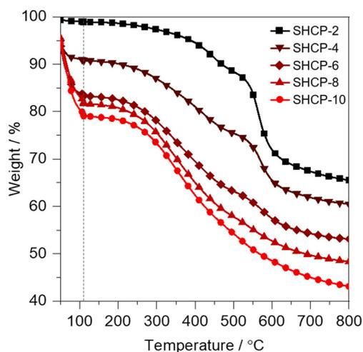
Fig. 3 Thermogravimetric analysis of SHCPs heated to  $800 \text{ }^\circ\text{C}$  in a  $\text{N}_2$  atmosphere. A 10 min isothermal step was included at  $110 \text{ }^\circ\text{C}$  to remove residual water (indicated by the vertical grey dotted line).
