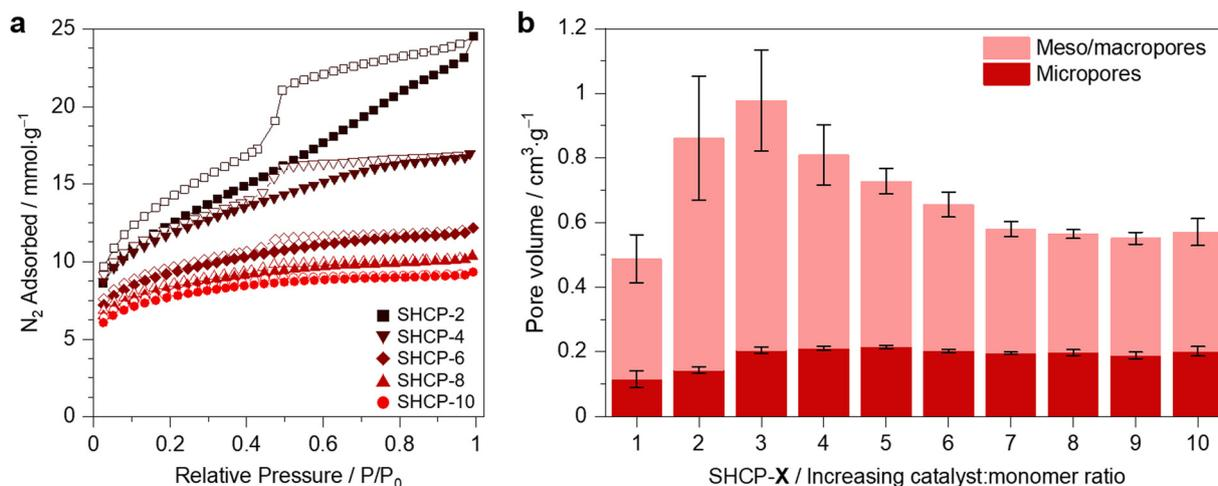
Fig. 2 Textural properties of SHCPs: (a)  $\text{N}_2$  adsorption–desorption isotherms for a selection of SHCPs, the remainder are shown in Fig. S4 (ESI†). Filled symbols represent adsorption and empty symbols represent desorption. (b) Pore volume of all SHCPs divided into micropore contributions (red) and mesopore/macropore contributions (pink).
