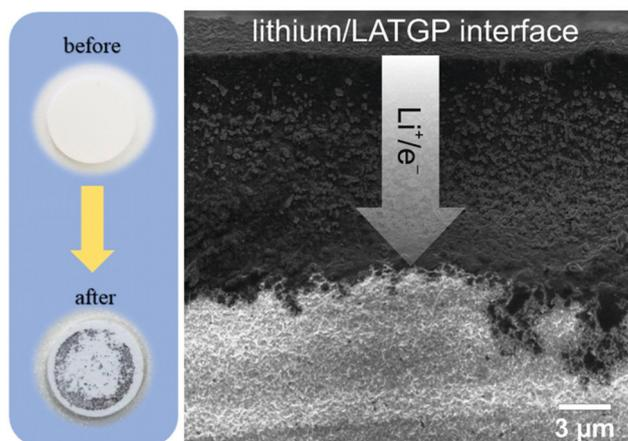
Fig. 1 LAMP pellets before and after the contact with the Li metal chip and SEM cross-section image of LATGP after contact with Li metal.<sup>75</sup>
