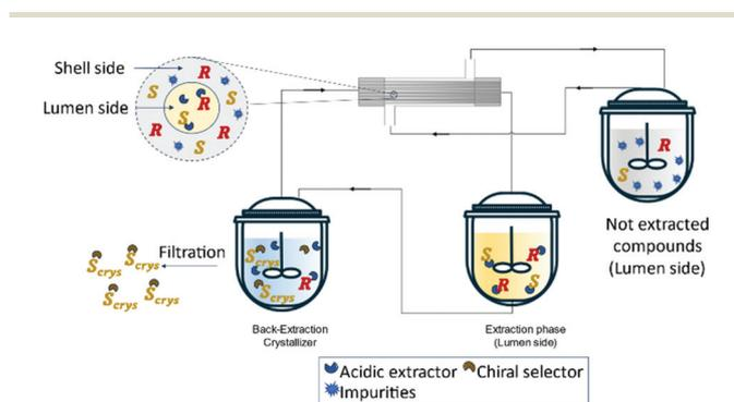
**Fig. 16** Schematic representation of a solution purification and enantiomeric separation. The lumen side contains an acidic extractor selective to the racemic compounds. The extracted solution is feed into the crystallizer where it contains a chiral selector that will form a salt with the (*S*)-enantiomer and precipitate as a crystal. Adapted from ref. 127.
