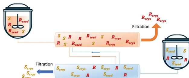
Fig. 7 Illustration of coupled plug flow crystallizer *via* mother liquor exchange. Adapted from ref. 91.
