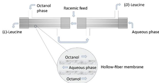
**Fig. 13** Separation of leucine enantiomers in a hollow fiber module. Shell side: octanol, lumen side: aqueous solution. Leucine enantiomers are collected in the exit streams of the module. Adapted from ref. 129.
