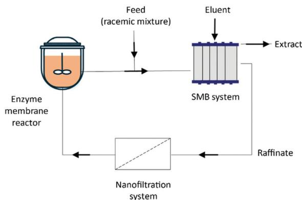
**Fig. 18** Integration of simulated moving bed chromatography, enzymatic racemization and nanofiltration to produce (D)-methionine. Extract: (D)-methionine solution; raffinate: (L)-methionine solution; nanofiltration system: concentration of the raffinate solution; enzyme membrane reactor: racemization of (L)-methionine.<sup>307</sup>
