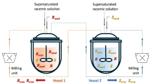
Fig. 5 Illustration of a simultaneous preferential crystallization with two vessels coupled *via* mother liquors exchange and milling units for large crystals breakage and fines dissolution. Adapted from ref. 65.
