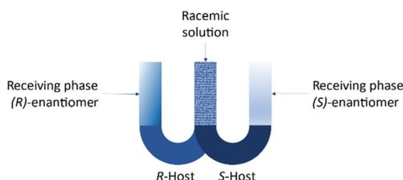
Fig. 11 Resolving machine developed by Cram *et al.*<sup>105</sup>
