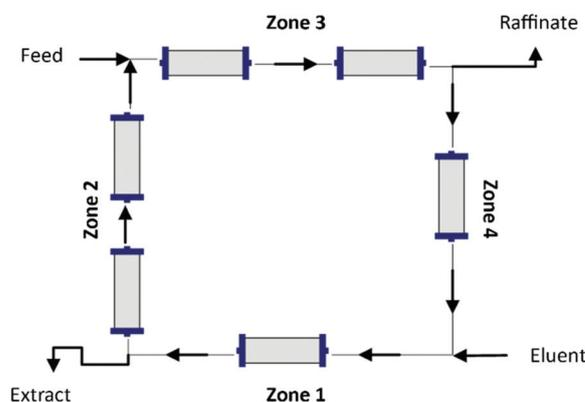
Fig. 17 Set-up for the separation of guaifenesin enantiomers by SMB process with [1-2-2-1] configuration. (feed: racemic solution of guaifenesin; raffinate: solution of (*R*)-guaifenesin; eluent: hexane/ethanol 70/30; extract: *S*-guaifenesin.) Adapted from ref. 301.
