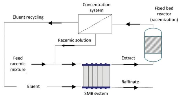
**Fig. 19** Integration of simulated moving bed chromatography, enzymatic racemization, and a concentration system to produce pure enantiomers. Extract: undesired enantiomer solution; raffinate: desired enantiomer solution; fixed bed reactor containing an immobilized enzyme to racemize the undesired enantiomer. Concentration system: concentration of the extract solution. Both streams (racemic solution and eluent) are recycled and feed into the SMB system.
