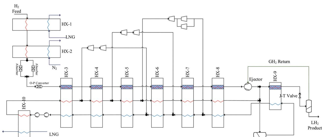
Fig. 9 Process block diagram for the Kuendig model. Simplifications have been implemented based on the original PFD: (i) N<sub>2</sub> compressor system and N<sub>2</sub> cold box are combined as HX-2; (ii) H<sub>2</sub> compressor system is represented by HX-10; two individual cold streams through HX3–HX7 are combined as one cold stream.
