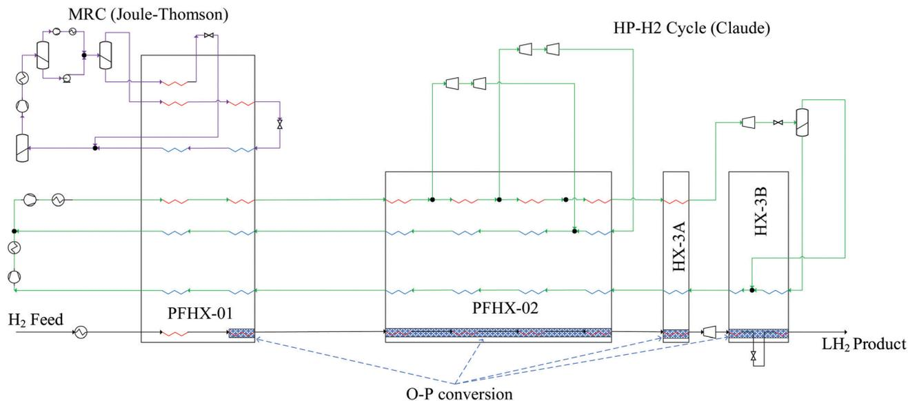
Fig. 10 Process flow diagram for the HP-H<sub>2</sub> Cycle model.
