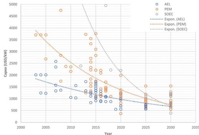
Fig. 6 Examples of CAPEX estimates for different electrolyser types for the year of development. Source: Glenk & Reichelstein.<sup>155</sup>
