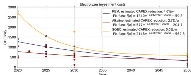
Fig. 7 Expected cost reductions to 2050 of AEC, PEMEC, and SOEC, based on data from PIK.<sup>154</sup>
