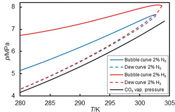
Fig. 11 Dew and bubble curves of impure CO<sub>2</sub> in comparison with the vapour–pressure curve of pure CO<sub>2</sub>. Equation-of-state model fitted to experimental data, adapted from ref. 206.
