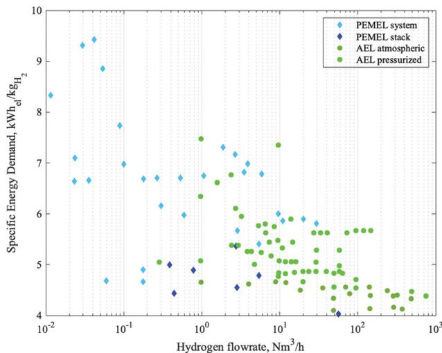
Fig. 5 The dependency of specific energy demand on the production rate today. Based on Smolinka.<sup>150</sup>
