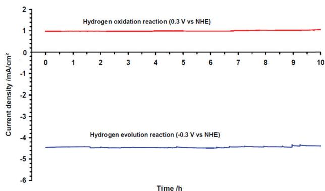
Fig. 137 Long-run electrolysis experiments for both hydrogen evolution and oxidation carried out respectively at  $-0.3$  and  $+0.3$  V vs. NHE in H<sub>2</sub>SO<sub>4</sub> (0.5 mol L<sup>-1</sup>) on a membrane electrode on which MWCNTs have been deposited and further Ni-functionalised. Reprinted with permission from ref. 1677 Copyright 2009 AAAS.
