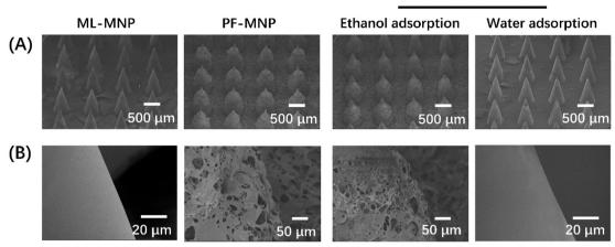
Fig. 2 SEM images of the overall (A) and partial (B) morphology of ML-MNP, PF-MNP, and PF-MNP after adsorbing ethanol and water.
