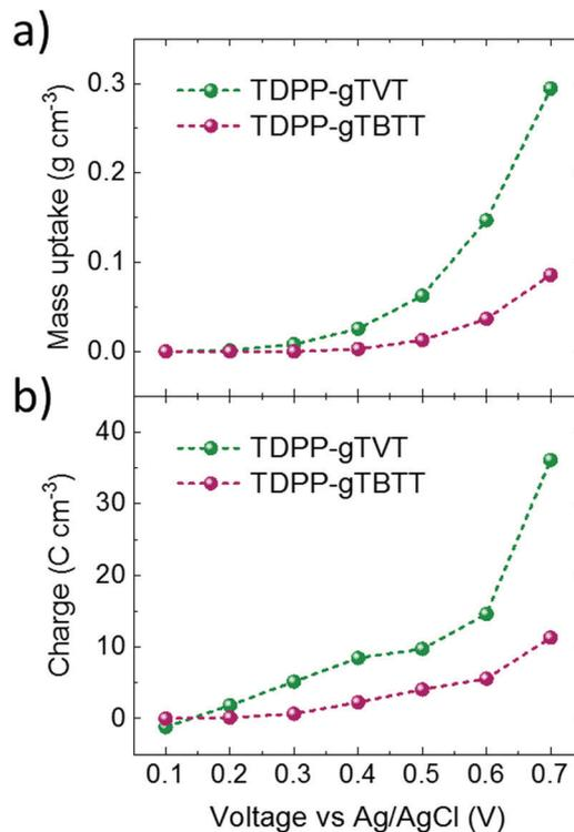
Fig. 3 Electrochemical quartz crystal microbalance with dissipation monitoring (EQCM-D) results of **TDPP-gTVT** and **TDPP-gTBTT**. The differences in (a) the electrolyte uptake and (b) charge generation per unit volume during the application of doping potentials from 0.1 V to 0.7 V vs. Ag/AgCl with a step of 0.1 V.
