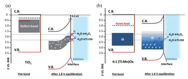
Fig. 5 Interfacial band energetics of semiconductive electrocatalysts. (a) "Leaky" TiO<sub>2</sub> and (b) 4:1 (Ti,Mn)O<sub>x</sub> films. The left panel of each diagram was drawn under flat band conditions, and the right panel of each diagram was drawn where the electrode was poised at  $+1.8 \text{ V}_{\text{RHE}}$  during water oxidation. Box height was drawn based on the estimated top edge of the Ti<sup>3+</sup>-defect band or the Mn<sup>3+</sup> intermediate band.
