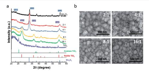
Fig. 1 (a) Grazing incident X-ray diffraction (GI-XRD) spectra and (b) plan-view scanning electron microscope (SEM) images of annealed (Ti,Mn)  $O_x$ . Samples denoted  $Mn_2O_3$  and  $TiO_2$  represent annealed ALD  $MnO_x$  and  $TiO_x$ , respectively.
