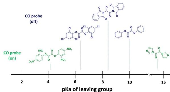
Fig. 3 Examination of the effect of pK<sub>a</sub> of the leaving group on the CO releasing capacity of 1,2-dicarbonyl compounds using a CO probe, COP-1.
