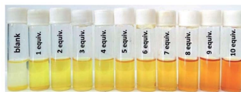
Fig. 15 Colorimetric detection behaviour of the HEPES suspension of \text{UiO-66}-(\text{NO}_2)_2 with increasing concentration of \text{Na}_2\text{S} in daylight. Reprinted with permission from ref. 95. Published (2018) by The Royal Society of Chemistry.
