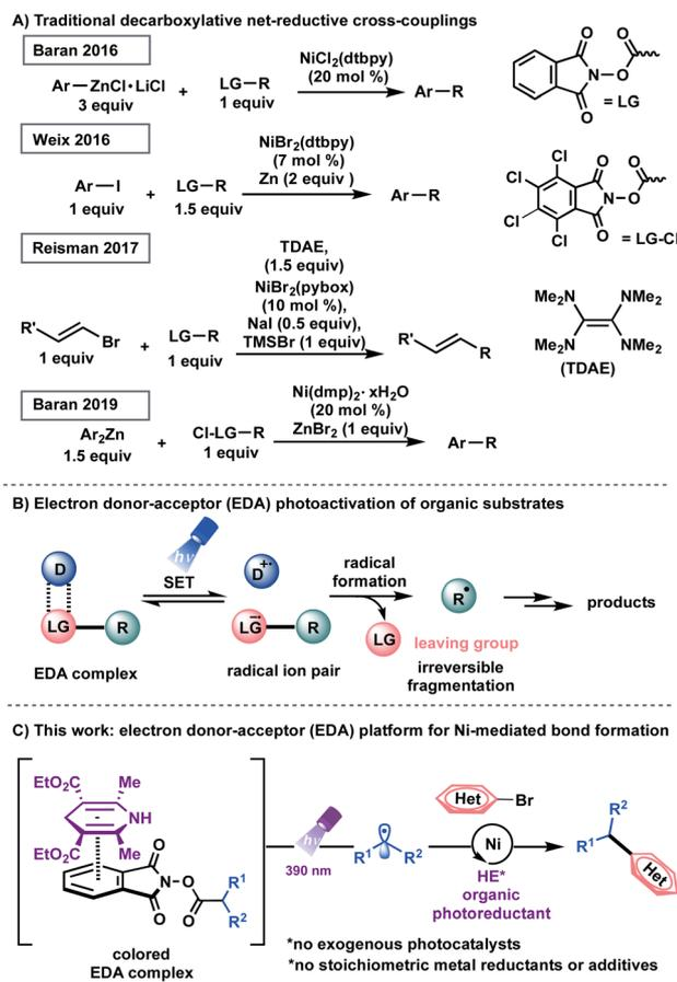
**Scheme 1** (A) Strategies toward net-reductive decarboxylative-based cross-couplings. (B) Overview of electron donor-acceptor (EDA) photoactivation. (C) Electron donor-acceptor (EDA) complex platform for Ni-mediated alkyl transfer using HE as an organic photoreductant.
