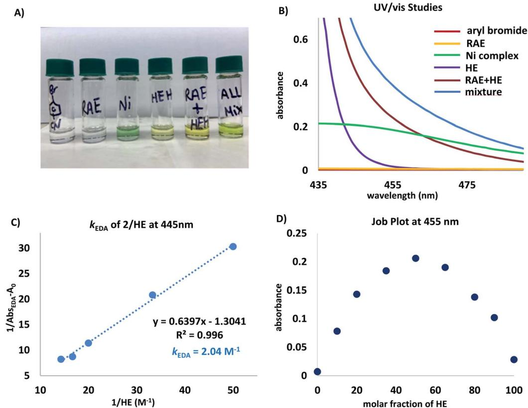
Fig. 1 (A) Visual appearance of reaction components and mixtures thereof. (B) UV/vis absorption spectra measured in DMA (0.1 M) unless otherwise noted. Ni complex = NiBr<sub>2</sub>(dtbpy), aryl bromide = 4-bromobenzonitrile, and RAE = cyclohexyl-*N*-hydroxyphthalimide ester. Mixture refers to a DMA solution of all reaction components. (C) Benesi-Hildebrand plot.<sup>28</sup> (D) Job plot<sup>29</sup> for a mixture of *N*-(cyclohexyl)-hydroxyphthalimide ester (**2**) and HE in DMA (0.2 M).
