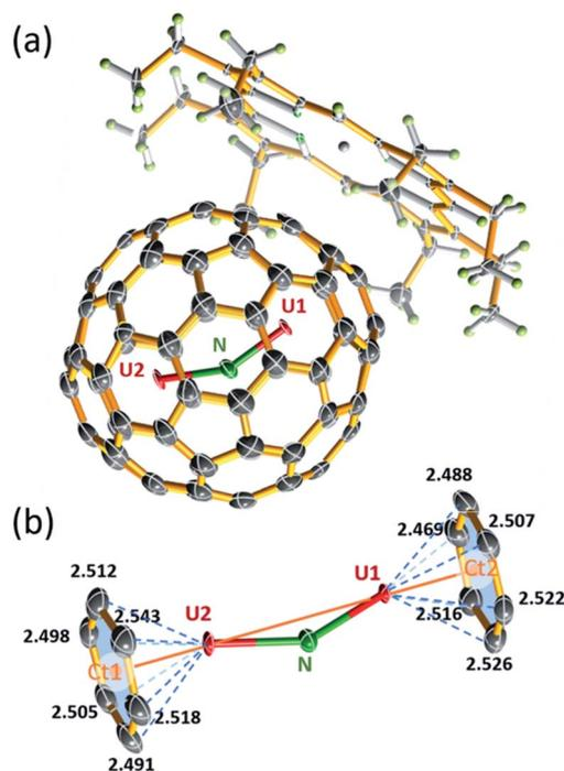
Fig. 2 (a) The ORTEP drawing of  $U_2N@I_h(7)-C_{80} \cdot [Ni^{II}-OEP]$  with 50% thermal ellipsoids. Only the major sites of the U atoms are shown, and the solvent molecules are omitted for clarity. (b) View of the relationship between the major UNU cluster and the closest cage portion (bond length in angstroms).
