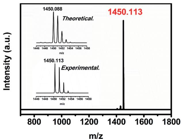
Fig. 1 The positive-ion mode MALDI-TOF mass spectrum of  $U_2N@I_h(7)-C_{80}$ . The insets show the expansions of the corresponding experimental isotopic distributions of  $U_2N@I_h(7)-C_{80}$  in comparison with the theoretical ones.
