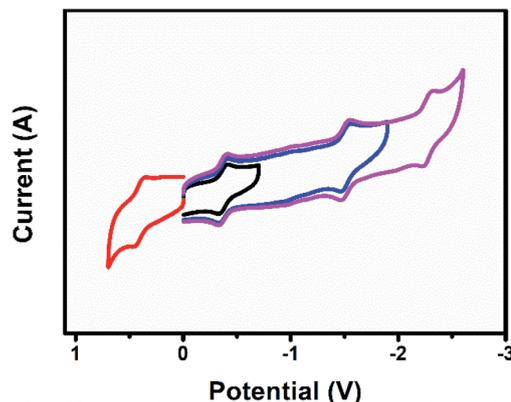
Fig. 8 Cyclic voltammogram of  $U_2N@I_h(7)-C_{80}$  in  $(n-Bu)_4NPF_6/1,2$ -dichlorobenzene.
