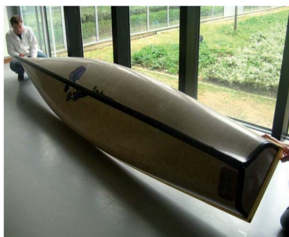
Fig. 2 Flax/PLA canoe manufactured during the NAVECOMAT project.
