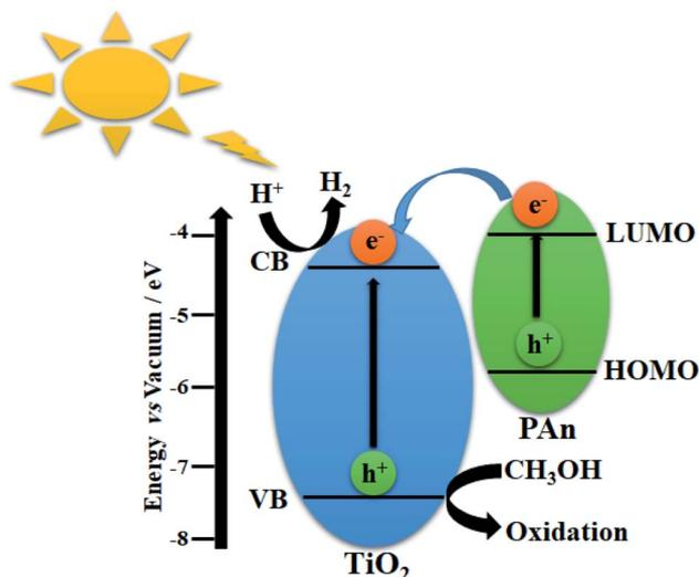
Fig. 16 Scheme illustrating the photocatalytic hydrogen production *via* water splitting over TiO<sub>2</sub>@PAN heterostructure.
