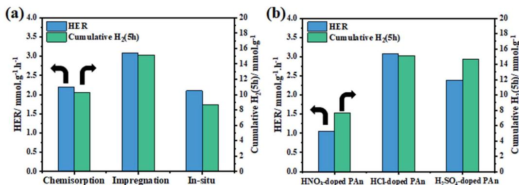
Fig. 9 The initial and cumulative (5 h) hydrogen evolution rate of (a) TiO<sub>2</sub>@5PAN composites fabricated by chemisorption, *in situ* polymerization, and impregnation methods and (b) TiO<sub>2</sub>@5PAN composites modified with various counterions, NO<sub>3</sub><sup>-</sup>, SO<sub>4</sub><sup>2-</sup>, and Cl<sup>-</sup>.
