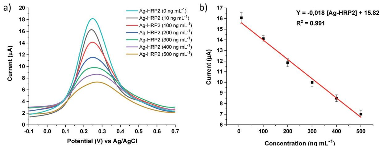
Fig. 6 a) DPV recorded with the Ab-PfHRP2/DHP/GE electrochemical immunosensor upon additions of Ag-PfHRP2 (10, 100, 200, 300, 400, and 500 ng mL<sup>-1</sup>), (b) calibration curve:  $Y = -0.018 [\text{Ag-PfHRP2}] + 15.82$ , with an  $R^2 = 0.991$ .
