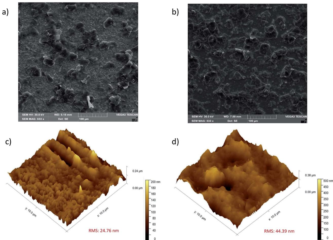
Fig. 2 SEM and 3-dimensional AFM images: (a and c) DHP/GE surface, (b and d) Ab-PfHRP2/DHP/GE surface.
