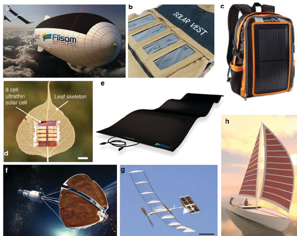
Fig. 1 Flexible solar cells and their diverse applications. (a) Solar-powered high altitude airship, 2 (b) solar vest, 3 (c) solar recharge backpack, 4 (d) solar leaf, 7 (e) flexible solar panel, 2 (f) flexible perovskite solar cells for space application, 5 (g) solar-powered model plane, 7 and (h) powering a boat with printed solar. 6
