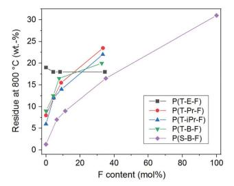
Fig. 7 Influence of the molar content of F units on the residue after TGA at  $800\,^{\circ}\text{C}$ .
