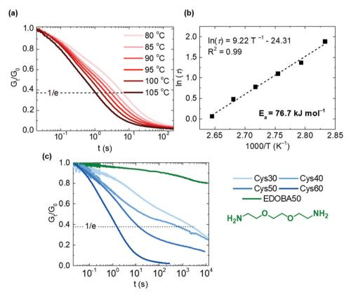
Fig. 4 Dynamic properties of the PA CANs; (a) stress relaxation curves of Cys60 at different temperatures, (b) relaxation times ( $\tau$ ) as a function of the temperature and calculation of the activation energy ( $E_a$ ) for Cys60 and (c) comparison of the stress relaxation of Cys30–60 at 100 °C.
