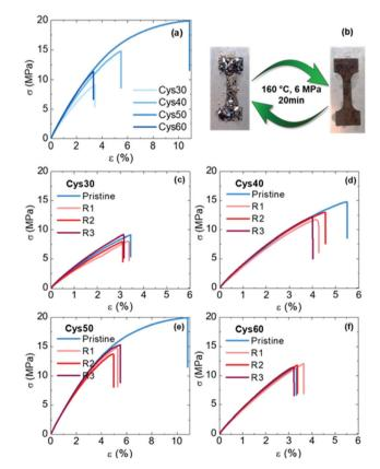
Fig. 5 Mechanical properties of the PA CANs; (a) stress-strain curves of the pristine networks, (b) appearance of a reprocessed sample after compression molding and (c-f) stress-strain curves of the reprocessed CANs.
