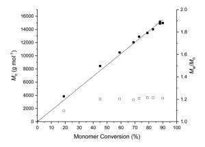
Fig. 1 Number-average molecular weight  $(M_n)$  and dispersity  $(D_M = M_w/M_n)$  plotted against monomer conversion for the ROP of ε-allyl-ε-caprolactone using Mg(BHT)<sub>2</sub>(THF)<sub>2</sub> and 4-methoxybenzyl alcohol as initiator ([ $M_0$ ]/[ $I_0$ ] = 50). Dispersity determined by SEC analysis in CHCl<sub>3</sub> (0.5% NEt<sub>3</sub>), calibrated against polystyrene standards.
