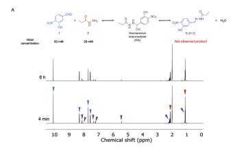
Fig. 2 (A) Reaction between aldehyde 1 and acylhydrazide 2 in  $CD_3CN$  to form acylhydrazone 3.  $^1H$  NMR (500 MHz, 288 K) spectra at different reaction times. Blue, red and purple arrows indicate the signals of compounds 1, 2 and HA, respectively.
