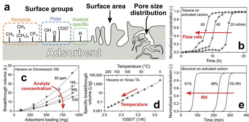
Fig. 2 (a) Critical adsorbent (filter) properties: surface chemical groups, surface area and pore size distribution. (b) Effect of overall flow rate through the filter on the breakthrough time.<sup>84</sup> (c) Effect of filter (adsorbent) loading and analyte concentration on breakthrough volume.<sup>85</sup> (d) Effect of temperature on specific breakthrough volume.<sup>80</sup> (e) Effect of RH on the breakthrough time.<sup>86</sup>
