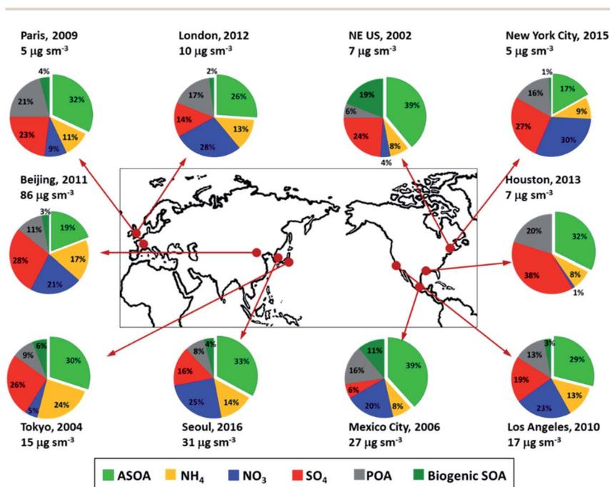
Fig. 3 Non-refractory submicron composition measured in urban and urban outflow regions from field measurements, all in units of μg m<sup>-3</sup> at standard temperature (273 K) and pressure (1013 hPa) (adapted from Nault *et al.*<sup>69</sup>).
