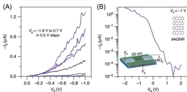
Fig. 13 (A)  $I_d$ – $V_d$  characteristics of the 9-AGNR FET. (B)  $I_d$ – $V_g$  of the device showing high  $I_{\text{on}} > 1 \mu\text{A}$  for a 0.95 nm wide 9-AGNR and a high  $I_{\text{on}}/I_{\text{off}}$  of  $\sim 10^5$ .<sup>197</sup> Copyright 2017. Adapted with permission from Macmillan Publishers Ltd: Nature Communications.
