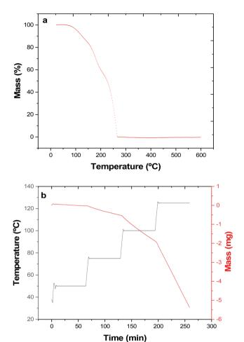
Fig. 1 (a) Thermogravimetric analysis of ["Bu<sub>3</sub>Sn(Te"Bu)] showing the percentage mass loss with temperature at a ramp rate of 5 °C min<sup>-1</sup> and a constant flow of argon gas. (b) Isothermal step TGA experiment of ["Bu<sub>3</sub>Sn(Te"Bu)] used for vapour pressure determination.
