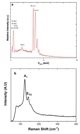
Fig. 3 (a) EDX spectrum highlighting the elements present within the SnTe film, the silicon present is attributed to the substrate. (b) Raman spectrum with the data highlighting the A<sub>1</sub> and E modes at 124 and 143 cm<sup>-1</sup>, respectively.<sup>1</sup>
