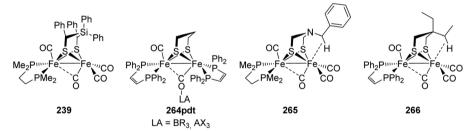
Fig. 79 Fe<sup>1</sup>Fe<sup>1</sup> models of the [2Fe-2S]-cluster exhibiting a rotated geometry
