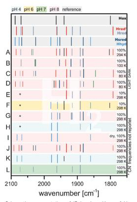
Fig. 11 Schematic representation of IR band positions of H2 reduced CrHydA1 (coloured background) in comparison with currently known states (grey background). IR signatures of known states are taken from Table 2. References for entries:  $A^{55}$   $B^{60}$  C and  $D^{82}$  E and  $F^{51}$  G to  $I^{75}$  J and K,67 L.72
