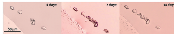
Fig. 9 Insulin crystals obtained with 0.1 M glycine in the vicinity of the 3-phase boundary (air, liquid and borosilicate cover glass) after 4, 7 and 14 days. As time passes by, existing insulin crystals promote the nucleation of more crystals (secondary nucleation).
