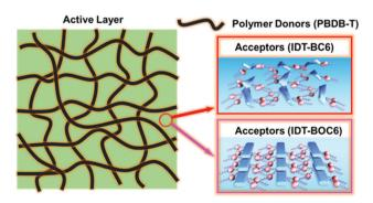
Fig. 9 Intuitive film morphology of PBDB-T:IDT-BOC6 and PBDB-T:IDT-BC6 blend films
