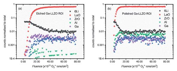
Fig. 5 ToF-SIMS depth profiles of etched (a) and polished (b) LLZO pellets, showing positive secondary ion species. Regions of interest (ROI) were selected based on areas without grain boundaries and pores in the etched and polished samples, respectively. The analysis was performed using 25 keV Bi<sup>+</sup> primary ions as the analytical beam and the sputtering was performed by 1 keV 300 nA O<sub>2</sub><sup>+</sup> beam (burst mode).
