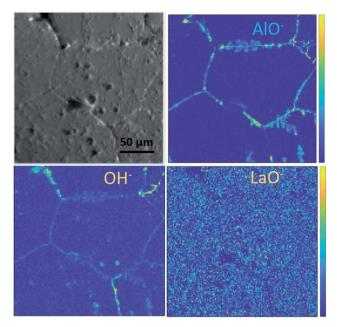
Fig. 7 ToF-SIMS negative secondary ion maps and optical image (greyscale) of an etched LLZO sample. The analysis was performed using 25 keV Bi $^+$  primary ions as the analytical beam and the sputtering was performed by 1 keV  ${\rm O_2}^+$  beam (burst mode).
