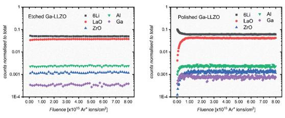
Fig. 3 ToF-SIMS depth profiles for etched and polished Ga-LLZO pellets, showing positive secondary ion species, operating under Bi<sup>+</sup> primary beam (25 keV) and  $Ar_n^+$  (13.5 nA) sputter beam conditions.
