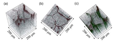
Fig. 8 Three-dimensional reconstruction with negative secondary ions of the etched Ga-LLZO sample. LaO<sup>-</sup> represents the bulk LLZO grains in dark green and OH<sup>-</sup> at the grain boundary surface in brown (a and b). The grain boundaries also contain AlO<sup>-</sup> in green (c).
