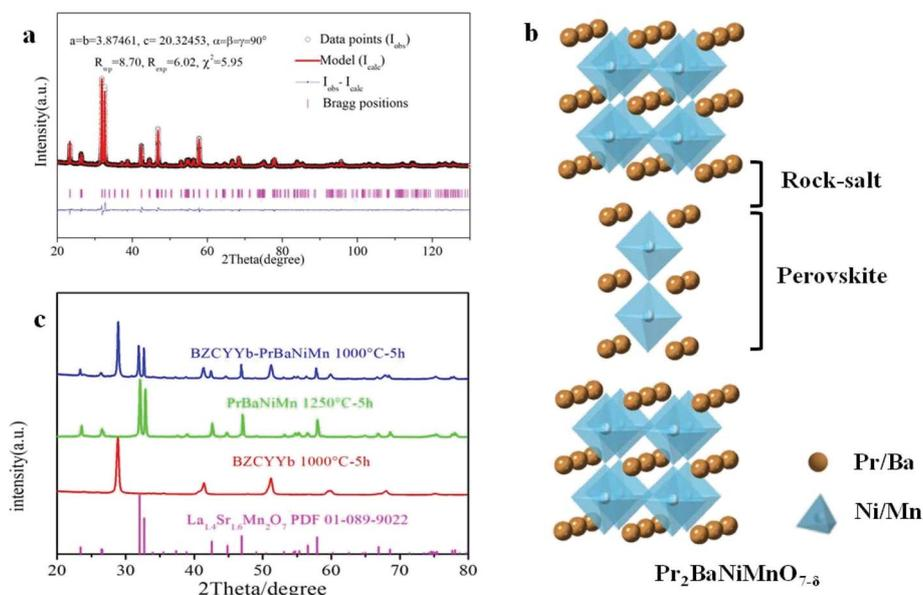
Fig. 2 (a) Rietveld refinement plot of PrBaNiMn powder using X-ray powder diffraction data,  $R_{wp}$  and  $\chi^2$  represent the weighted profile factor and reduced chi-square; (b) the crystal structure of  $Pr_2BaNiMnO_{7.8}$ ; (c) XRD patterns of PrBaNiMn, BZCYYb fired at 1250, 1000 °C and the dry-mixed composite powder BZCYYb–PrBaNiMn (5 : 5) fired at 1000 °C for 5 h, respectively.
