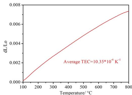
**Fig. 7** The thermal expansion coefficient of PrBaNiMn over the temperature range of  $100\text{--}800\text{ }^\circ\text{C}$ .
