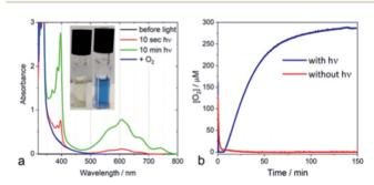
Fig. 2 (a) Spectral changes induced in an Ar-purged solution of nano-PDPB,  $100~\mu M~MV^{2+}$ , 10%~TEOA in MeCN by illumination with blue light and after aeration (inset: formation of the blue  $MV^{++}$  radical). (b) Time courses of oxygen evolution from water measured by a Clark electrode. Blue curve: with nano-PDPB (synthesized in mesophases) and red curve: no irradiation.
