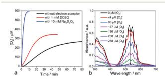
Fig. 4 (a) Time courses of oxygen evolution from water measured by a platinum Clark electrode in the absence of an electron acceptor (black) and in the presence of DCBQ (red) and S<sub>2</sub>O<sub>8</sub><sup>2-</sup> as electron acceptors (blue). (b) Titration of H2O2 with KMnO4 at different concentrations of photoproduced O2 in the absence of an electron acceptor.
