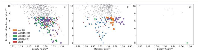
Fig. 10 ESF map of electron mobility in the predicted crystal structures of molecules (a) 4A, (b) 7A and (c) 2B. Each point corresponds to a distinct predicted crystal structure. Colouring and size of the circles correspond to the magnitudes of the calculated mean electron mobilities (in cm<sup>2</sup>  $(Vs)^{-1}$ ). Grey points are structures above 7 kJ mol<sup>-1</sup>, for which mobilities were not calculated.
