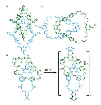
Fig. 23 (a) Geerts' bis(aryl bromide) functionalised octaamide [2]catenane, used to prepare main chain poly[n]catenanes through palladiumcatalysed cross couplings; (b) Kern, Sauvage and Geerts' bis-phenanthroline catenane with alcohol functionality used in polyesterification reactions: (c) Takata's heterocircuit [2]catenane with dienophile and masked-diene functionality for Diels-Alder polymerisation.
