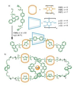
Fig. 7 Combining non-covalent templates with the CB[6]-catalysed azide–alkyne cycloaddition: (a) Stoddart's synthesis of a heterocircuit [4] rotaxane with  $\beta$ - and  $\gamma$ -CDs, and (b) Au-Yeung's [6]catenane synthesised using a Cu(i)-phenanthroline PMT.
