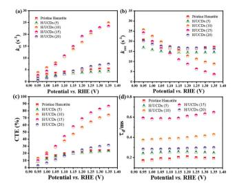
Fig. 7 (a)  $k_{\rm tr}$ , (b)  $k_{\rm rec}$ , (c) charge transfer efficiency (CTE), and (d) diffusion lifetime of the photogenerated charge carriers calculated from IMPS plots.
